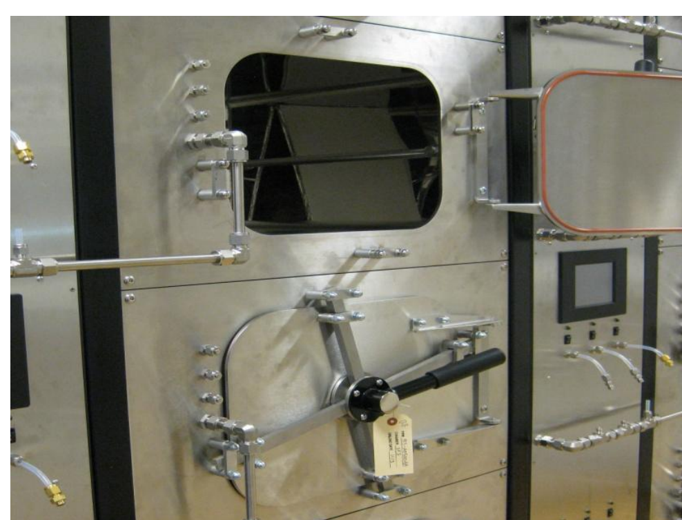
Dynamic Environmental Chamber used for emissions testing for building materials such as drywall
