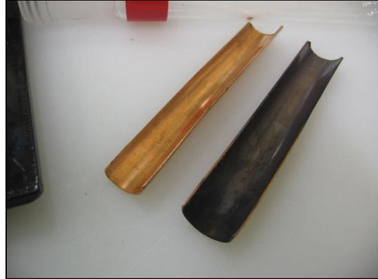
Subsequent scanning electron microscopy (SEM) with Elemental Energy Dispersive Spectroscopy (EDS) testing was done by the Major Analytical Instrument Center (MAIC) of the Department of Material Science & Engineering (MSE) at the University of Florida (Gainesville, FL), under the supervision of Dr. Amelia Dempere, PhD Laboratory Director, which confirmed high sulfur corrosion product on the Chinese copper sample.
