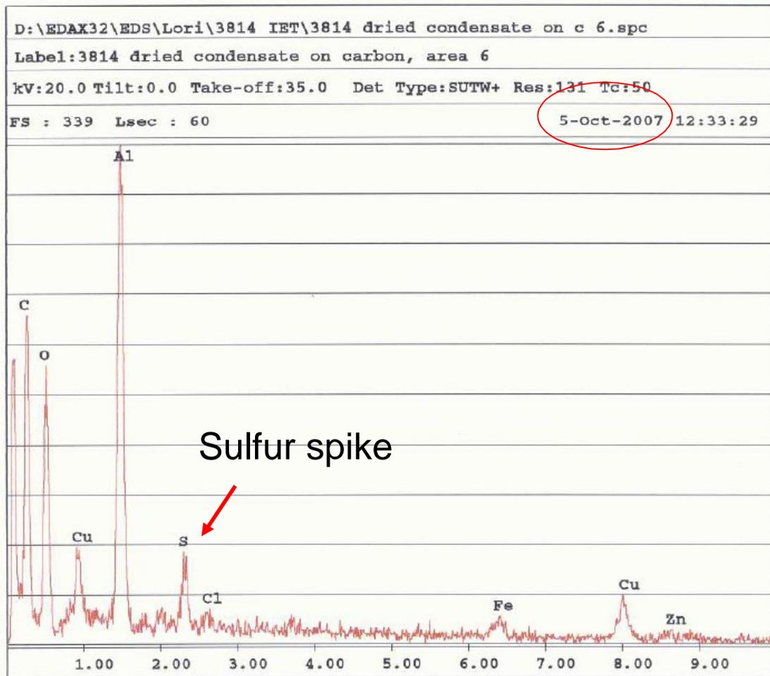
The condo development where these samples were taken has been determined to have contained Chinese Drywall and suffer from CDS. While coil failures were not unheard of in 2007, a specific building material such as Chinese drywall had not been implicated.
