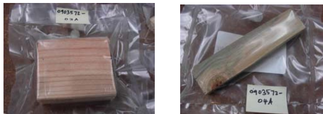
Photos of wood samples in evacuated 1L Tedlar bags.
