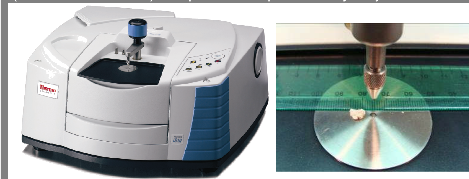
FIGURE 1. Nicolet iS10 FT-IR with ITR Smart Accessory for rapid analysis based on ATR (Attenuated Total Reflectance) with expansion of a sample and the Analyzer Crystal
